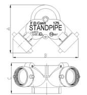
An exposed auxiliary inlet connection with 500G.P.M inlet capacity to supplement fire protection water supply. Exposed design provides an economical method of satisfying Fire Dept. inlet requirements.
